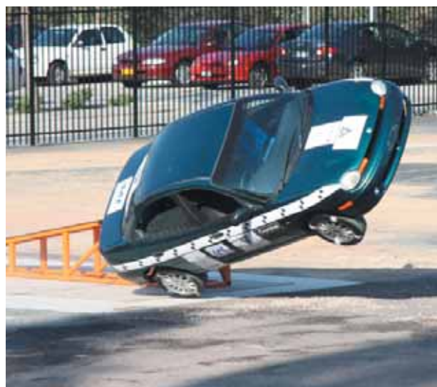
A vehicle undergoing the 'cork-screw' vehicle roll-over test, developed by the Crashlab for the 'Rollover Crashworthiness Symposium' in October 2008.
